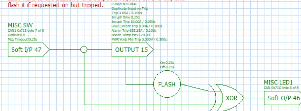
This is how you dim the keypad LEDs. The input here is from the "Lighting Example" page lighting enabled. If you manage one keypad from each PDU then you need one KP DIM in each PDU schematic, probably using soft inputs and outputs to share and agree the overall headlight state between PDUs.
