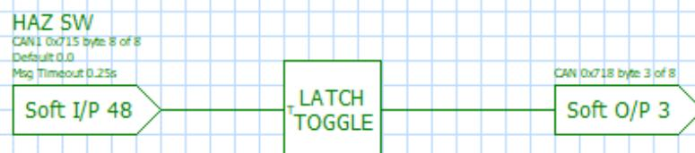
Here we receive that soft output back in (!!!) as a soft input as it came from another PDU, then send it back out to drive a keypad LED. If you want both keypads to be able to turn the hazards on and also light both LEDs you can toggle and share the switches like this (one PDU managing each keypad) then put an OR in each PDU to drive the appropriate LED on the keypad it is managing.
