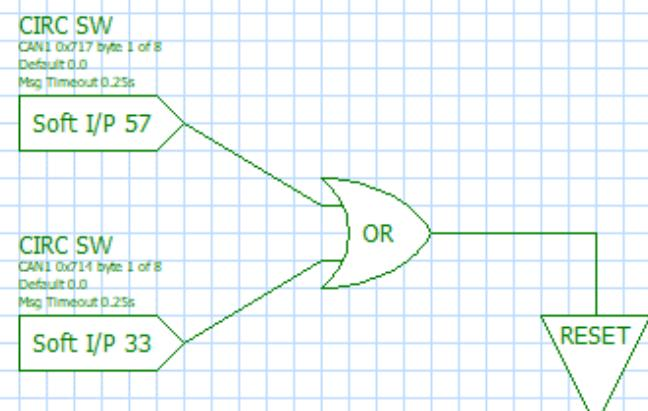
This is how to use the fault component to turn on the circuit reset button LED on both keypads, when both keypads are managed by the same PDU. With two PDUs managing a keypad each you would send the fault states in each to a soft output to send to the other PDU and then use an OR to set the keypad LED when either we are faulted or the other PDU is saying it is.
