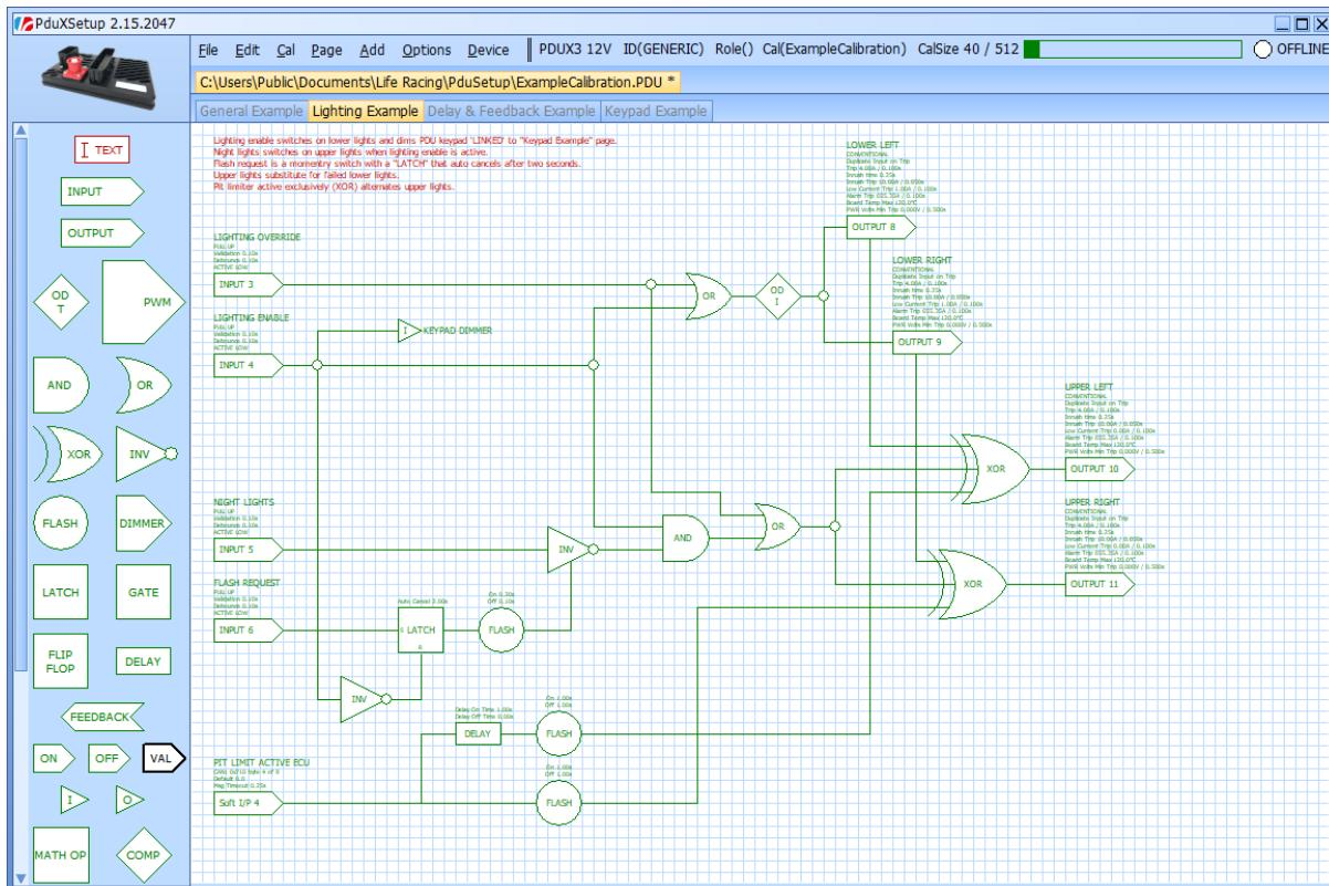
In the menu bar, the total calibration size and connection state is shown. The bar displayed represents the calibration size as a proportion of total available memory. A maximum of 512 logic components are allowed within a .pdux calibration. When this limit is surpassed, the bar will turn yellow and programming will not be allowed.
