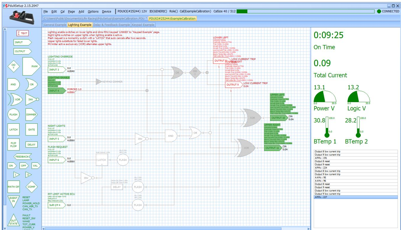
In this mode, components will become locked so they cannot be moved or edited. Input and output states as well as internal logic can be monitored. Inputs and outputs can be forced into on or off states by right clicking to bring up the options. Selecting automatic will revert the component to display real time states.
